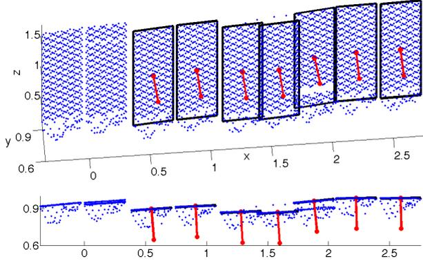
**Figure 12:** Point cloud of frames in 3D and top view with extracted planes of some frames
