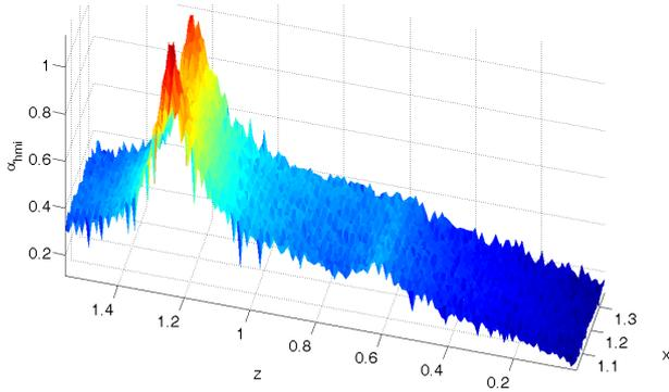
**Figure 8:** 2D scan of a wall fragment using the AC sensor. A horizontal power line is detected at  $y \approx 1.25$  m as shown by the peaks in the scan
