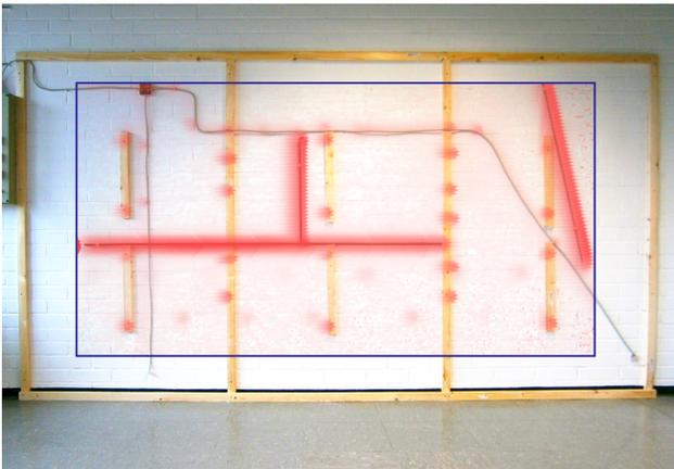
**Figure 16:** Picture of the wall with overlaid inductive scan results (highlighted by a frame)
