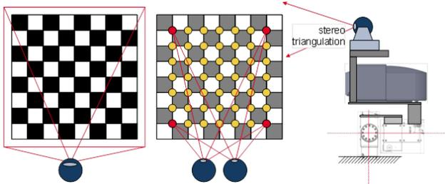
**Figure 3:** Estimation of the robot's orientation
