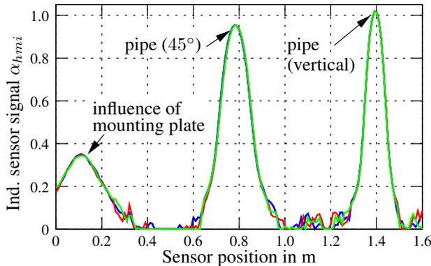
**Figure 5:** Inductive sensor data; different colors indicate different runs
