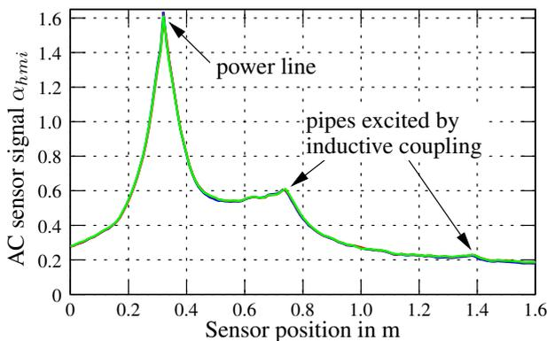
**Figure 6:** Alternating current sensor data (detection of a power line). Plots show high reproducibility.
