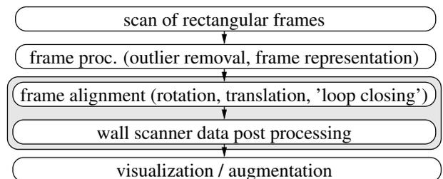
**Figure 11:** Flow chart of mapping procedure
