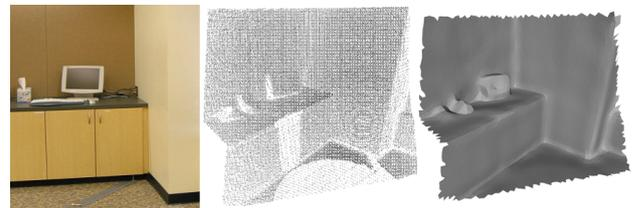
**Figure 7:** Left: Room corner. Middle: 3D Point Cloud. Right: Reconstructed Surface Mesh
