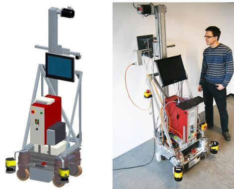
**Figure 4:** Mobile scanning system
