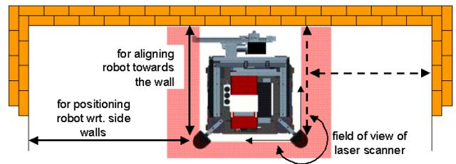
**Figure 10:** Top view on robot: Positioning and alignment of robot is based on laser scanners
