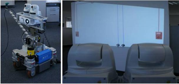
**Figure 1:** Left: Demonstrator for projection of in-wall information (mobile platform with traversable projector). Right: No distortion despite oblique projection
