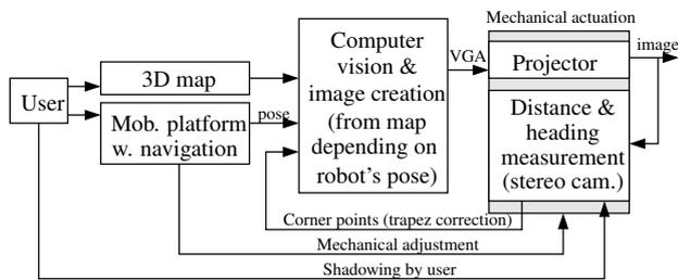
**Figure 2:** Basic concept for augmentation
