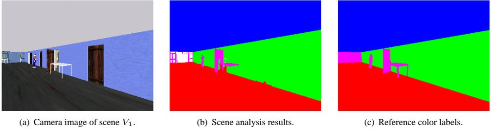
Figure 8: Scene analysis of the virtual reality scene  $V_1$ . The 2D regions corresponding to the detected objects are color-labeled in (b). (c) shows the manually labeled image used as reference. The overall recognition rate for this scene is 96.75%.
