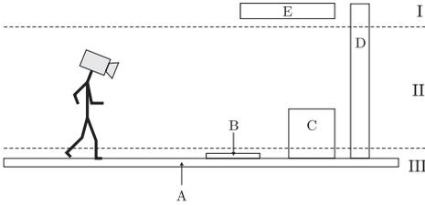
Figure 6: Categorization of scene objects by their spatial position. Only objects that are completely or partially in region *II* are navigation obstacles.
