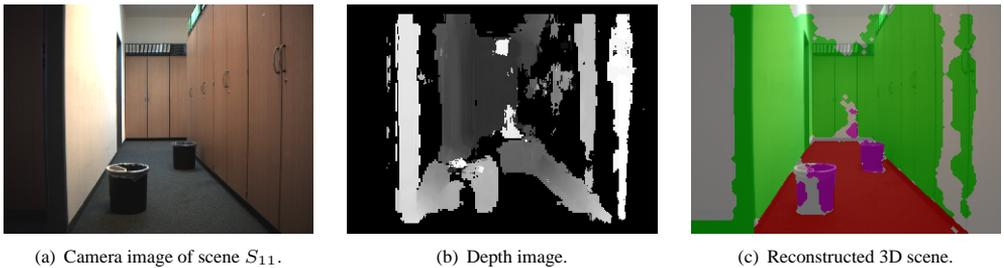
Figure 10: Scene analysis of the virtual reality scene  $S_{11}$ . The depth image in (b) is sparse, due to homogeneous textures on the floor and walls. With our knowledge-based approach, we are able to partially reconstruct those areas as demonstrated in (c). The overall recognition rate for this scene is 76.68%.
