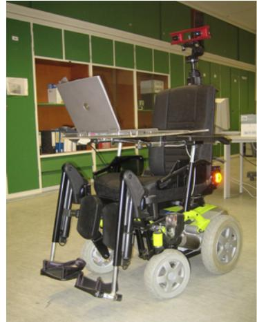
Figure 1: A *STORM*<sup>3</sup> wheelchair equipped with a stereo vision system used for assisted and autonomous navigation.
