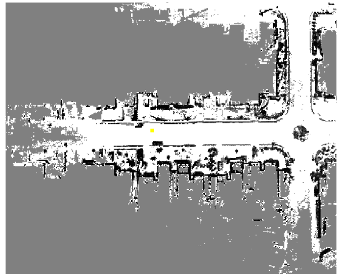
Fig. 3. Example for the evidence mapping of 3D lidar data onto a 2D grid. Darker spots correspond to high evidence for an obstacle while white cells correspond to drivable area. Unknown cells are marked as grey.
